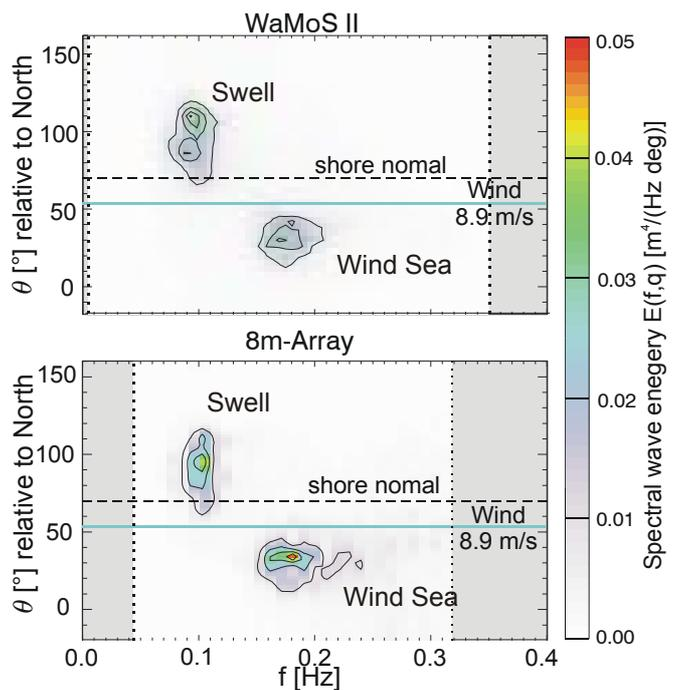
Figure 4: Sample of directional frequency wave spectra as obtained by 8m-Array (top) and WaMoS II (bottom) on Sept. 24th, 2005, 18:00 UTC.
